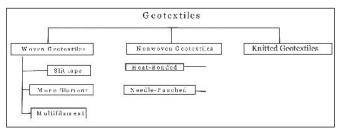
Geo textiles are generally made up of woven, nonwoven and knitted type of fabrics.
